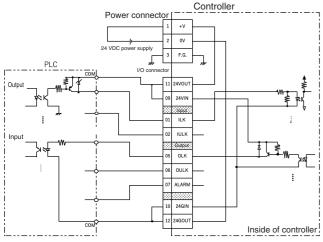
\* Even when using just input or output, short circuit 09-11 and 10-12.
