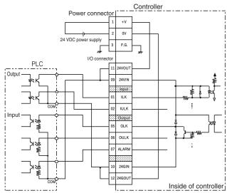
\* Even when using just input or output, short circuit 09-11 and 10-12.
