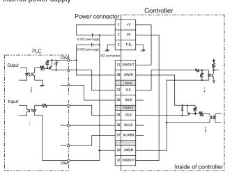
\* Even when using just input or output, connect power to 09 and 10.
